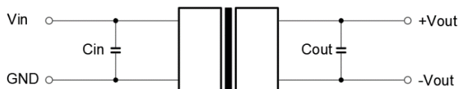
Figure 1. Typical external circuit
