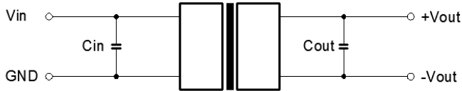
Figure 1. Typical external circuit
