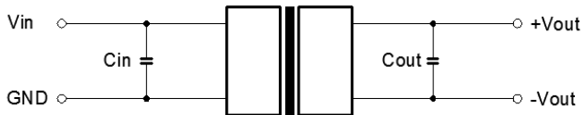
Figure 1. Typical external circuit
