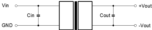
Figure 1. Typical external circuit
